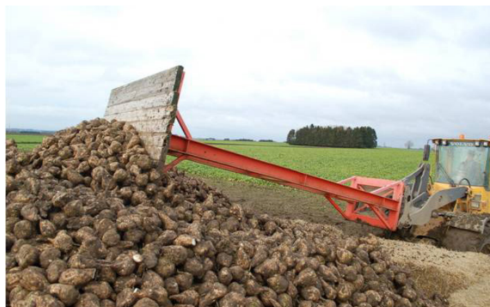
Figure 5.1: Equipment to make the sugar beet clamp domed and pit-free. (Photo: NBR).
