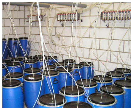
Figure 3.1: Equipment used at IRBAB for measuring the respiration losses from sugar beet during storage. (Photo: IRBAB).
