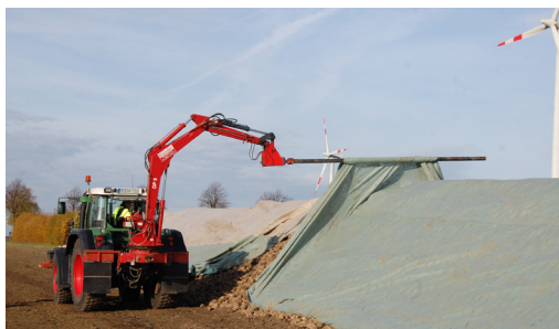
Figure 5.4: Mechanical covering of a sugar beet clamp and securing of the fleece. (Photos: Nordzucker).
