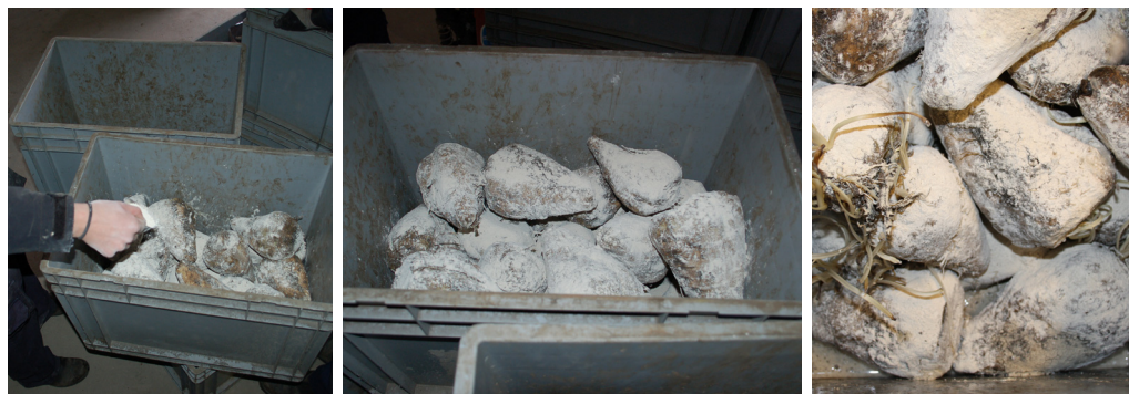
Figure 4.14: Storage trial with sugar beet treated with lime in amounts corresponding to 1% of beet weight. (Photos: NBR).
